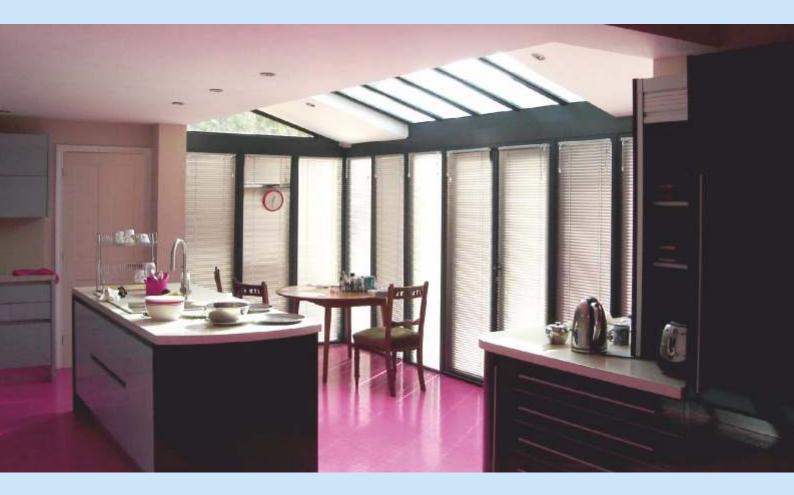
The superior natural strength of aluminium allows for a much larger glazed area with the structural integrity and strength to take several inches of snow and wind speeds of more than 100mph. This roof system is an energy efficient thermally broken system that is suitable for both commercial and domestic purposes.
